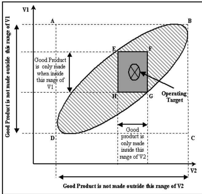
Figure 1 The Operating Zone in 2 dimensions
