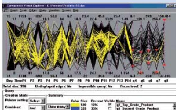
**Figure 1 (top):** The quality specifications for top-grade product are shown as red triangles, with all lines passing through all these 'top spec' areas coloured yellow, from which the process envelope can be derived
