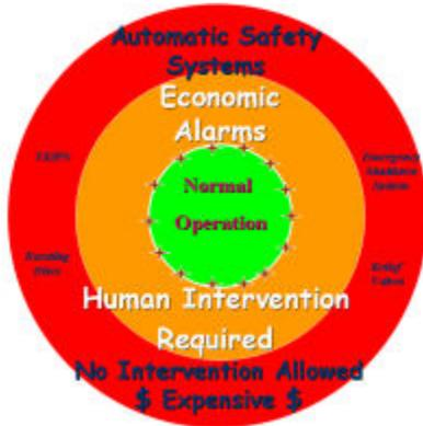
Figure 1 Alarm Limits as they are imagined to be
